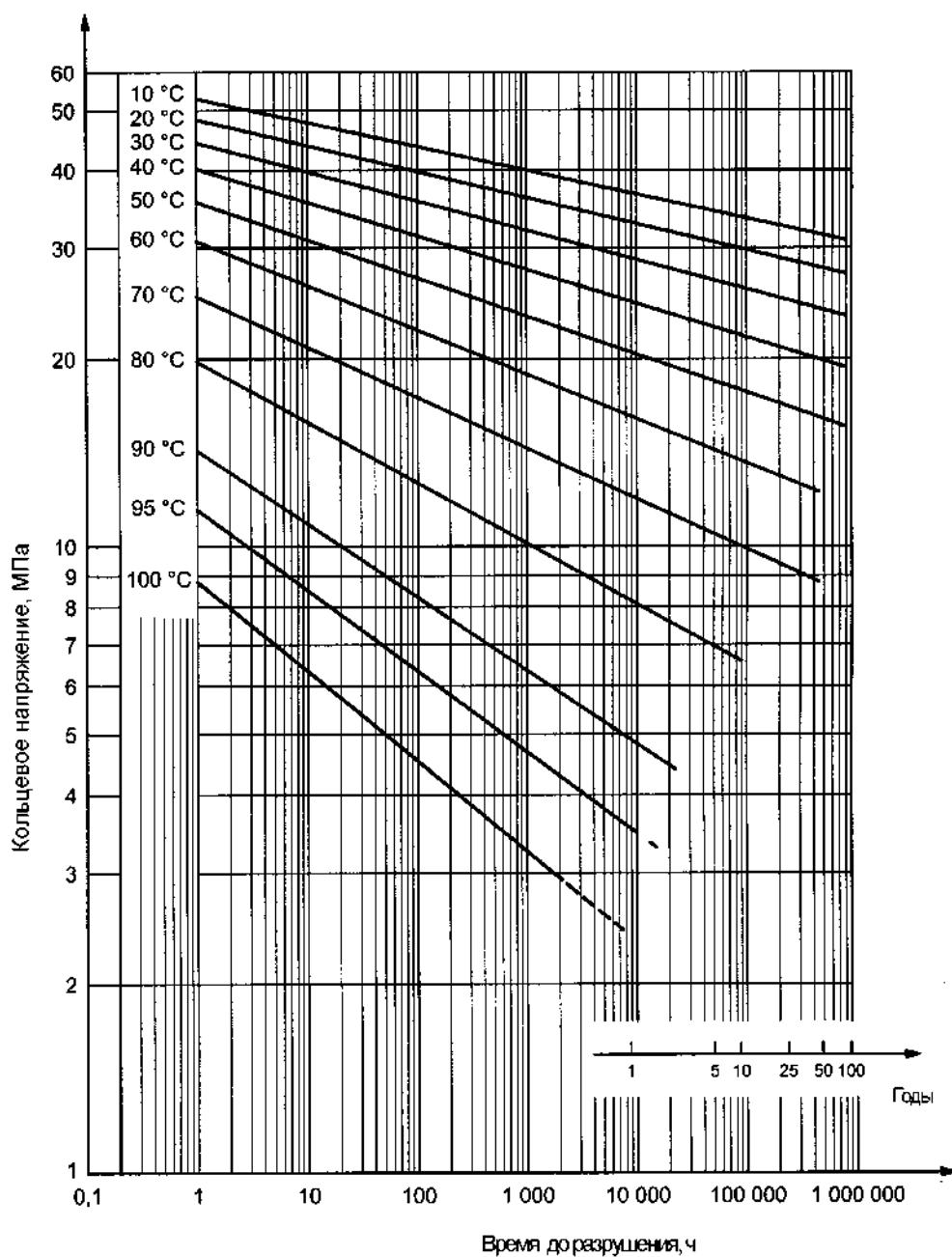
$$\lg t = -115,839 - \frac{22980}{T} \lg \sigma + \frac{45647,94}{T} + 54,73219 \lg \sigma,$$
