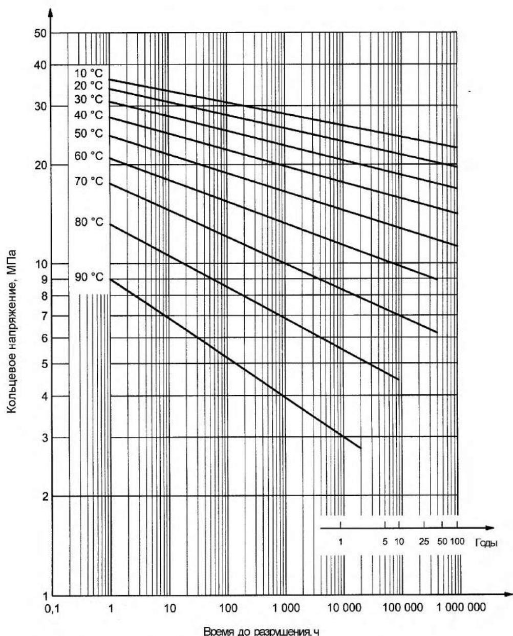
$$\lg t = -121,699 - \frac{25985}{T} \lg \sigma + \frac{47143,18}{T} + 63,03511 \lg \sigma,$$
