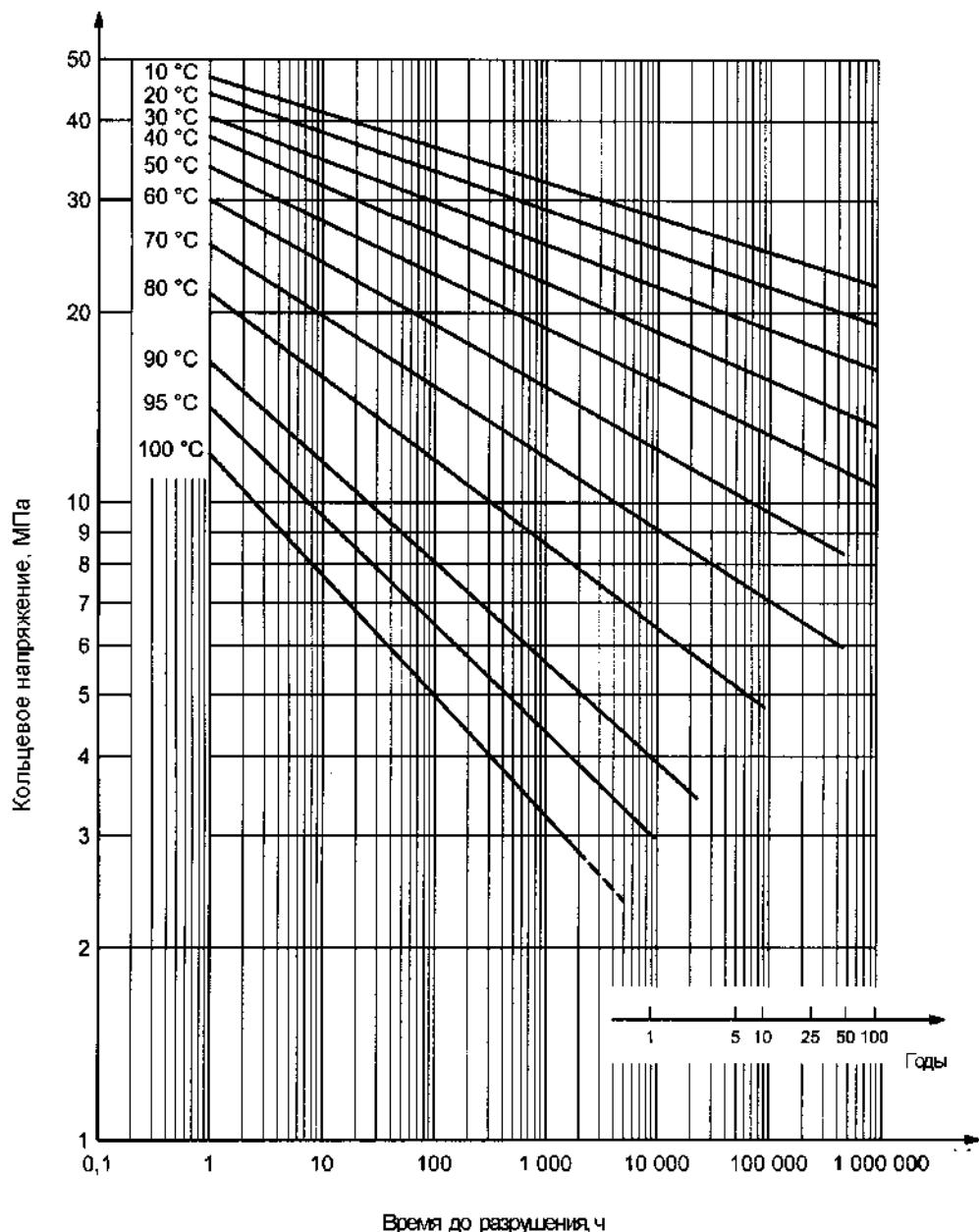
$$\lg t = -72,6624 - \frac{15253}{T} \lg \sigma + \frac{29245,14}{T} + 35,54 \lg \sigma,$$
