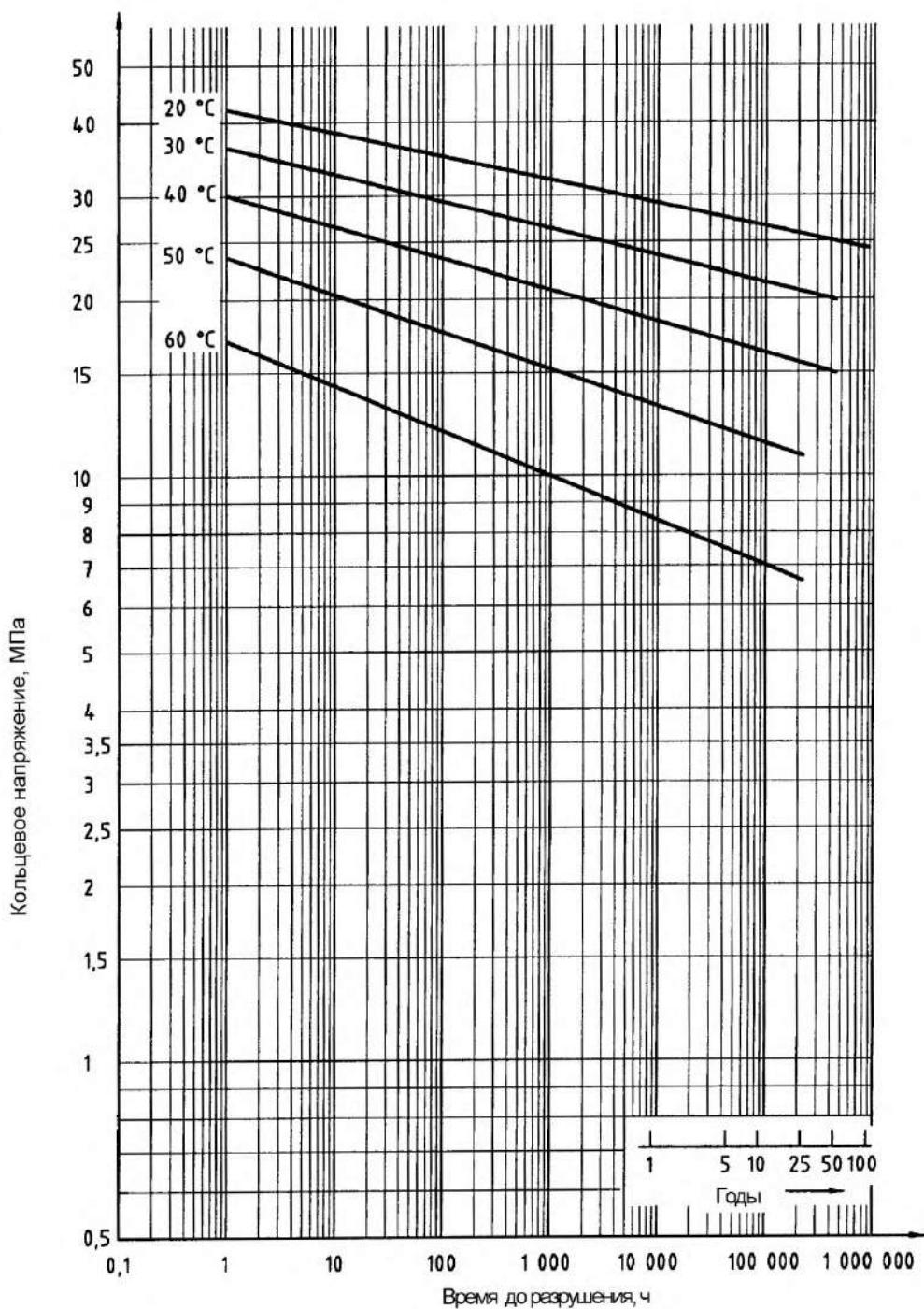
$$\lg t = -164,461 - \frac{29349,493}{T} \lg \sigma + \frac{60126,534}{T} + 75,079 \lg \sigma,$$
