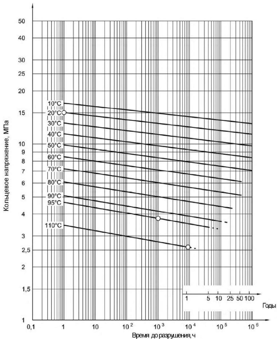
$$\lg t = -119,546 - \frac{23738,797}{T} \lg \sigma + \frac{52176,696}{T} + 31,279 \lg \sigma$$
