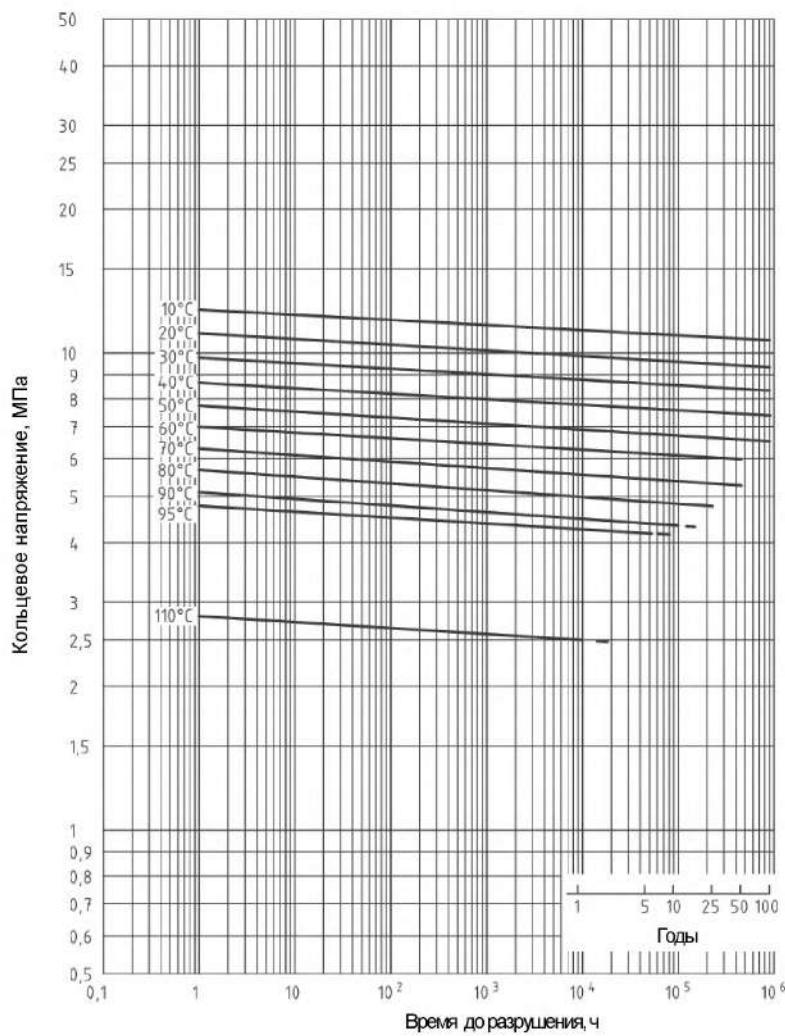
$$\lg t = -105,8618 - (18506,15/T) \lg \sigma + 57895,49/T + 24,7997 \lg \sigma,$$
